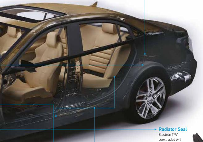
Elastron TPV coextruded with PP dampens the noise around the radiator and provides long term heat and chemical resistance.
